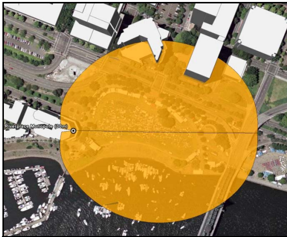
12 dBi gain (ANT-82) 90 degrees horizontal beamwidth 10 degrees vertical beamwidth
